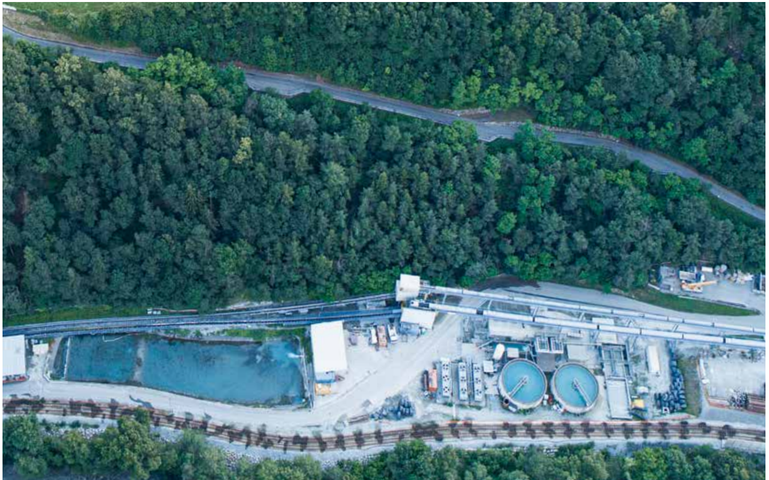
All water flowing from the tunnel during the construction phase is purified in the water treatment plants.
