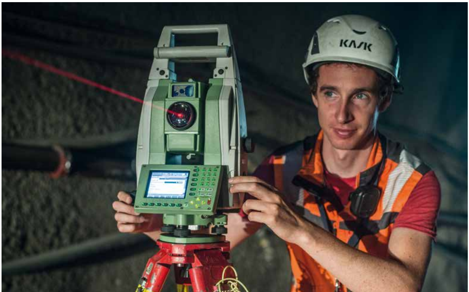
Surveyor at work with a tachymeter.
