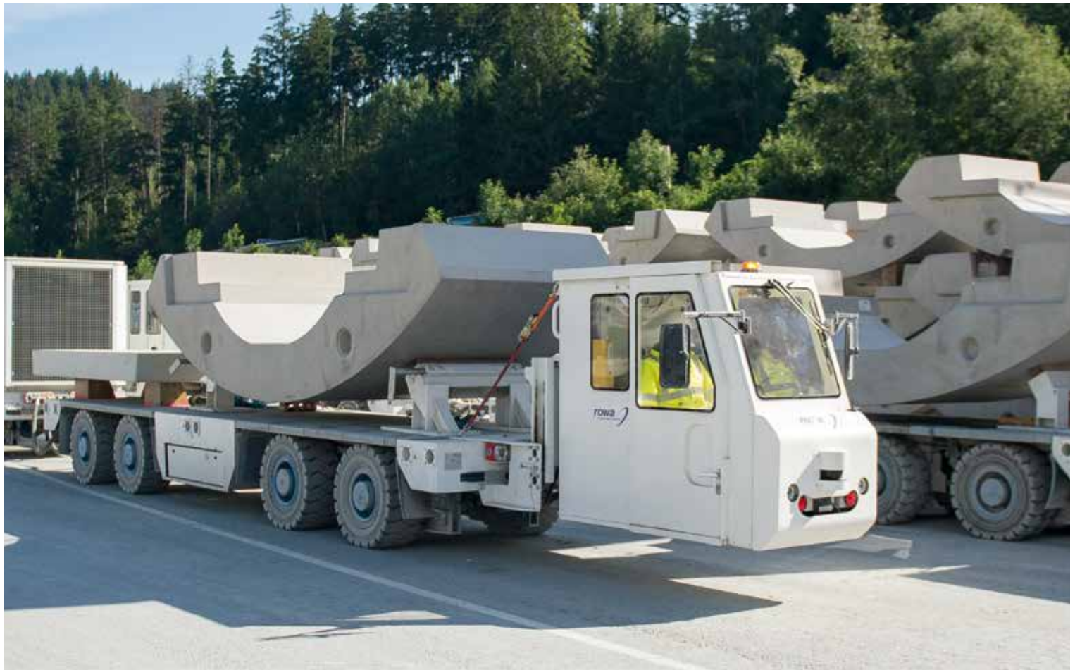
The so-called Multiservice Vehicle was used to supply the TBM in the Ahrental-Pfons exploratory tunnel.
