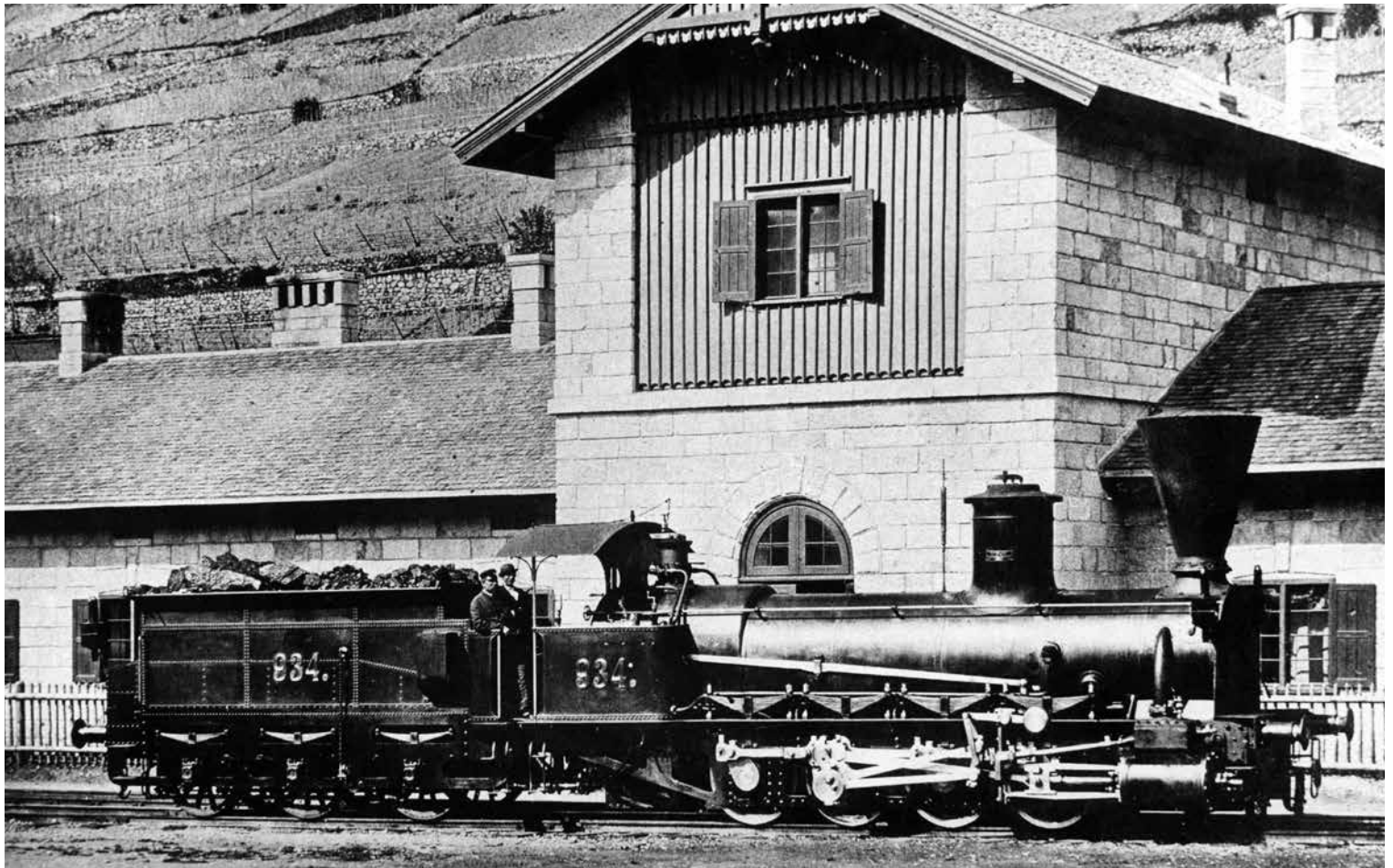
A SB 34 steam locomotive at Brenner station, put into service in 1867 – at the time, it was the heaviest and strongest locomotive in Austria. (Collection from the Verkehrsarchiv Tirol)
