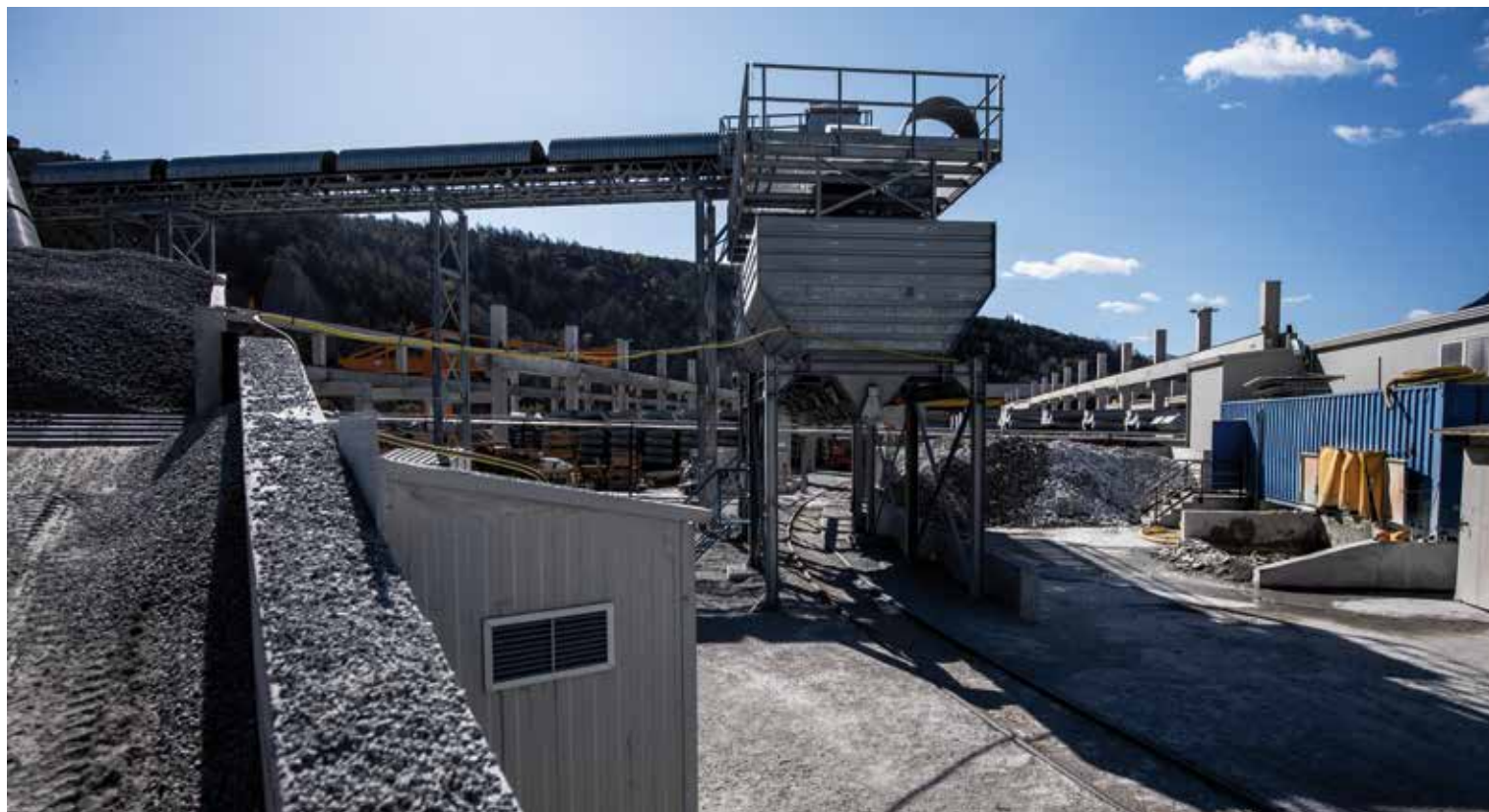
Most of the tunnel spoil is transported on conveyor belts.
